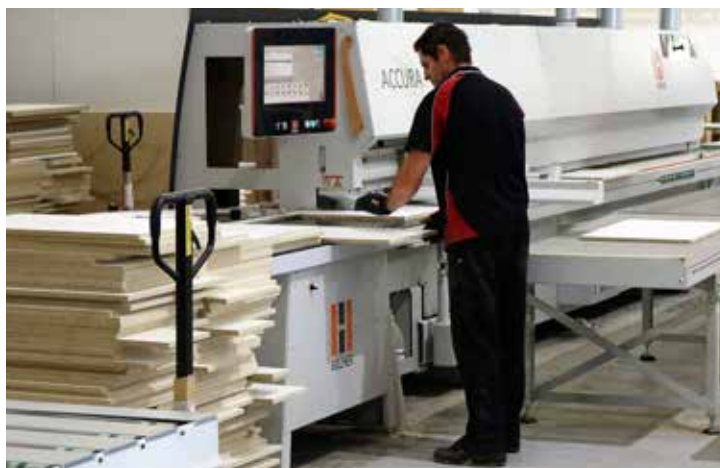
Phil Snowden operates Janper's recently installed Holzher Accura edgebander.
