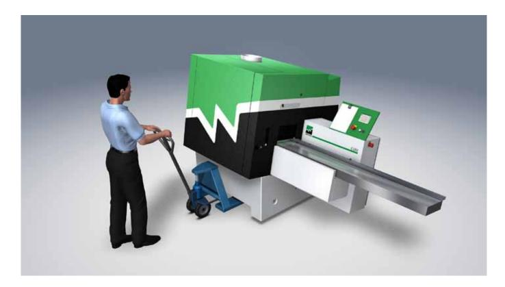
The Cube reinvents the planing operation. It is very fast, highly accurate and easy to use as never before, being equipped with new technology laser measuring and automatic adjustment for width and height. It is particularly suitable for smaller companies and those that currently use standard machines and traditional methods of 4-sided planing. It does not have to be run all day long to be profitable – as it is so productive, efficient and attractively priced.
