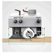
Pressure elements and extraction hood can be adjusted very simply to suit the cutting circle of each tool. This guarantees a comfortable setup and sure guiding of the workpieces.
