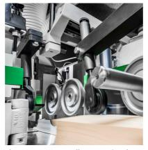
The top pressure roller opposite the left spindle only needs to be adjusted to the tool cutting circle once. When changing the width of the workpiece, the roller moves with the left spindle!
