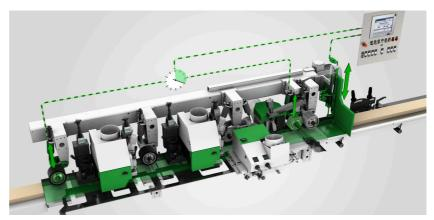
The workpiece monitoring automatically detects whether there is a workpiece inside the machine or not. This allows dimensional changes while the machine is running. You benefit from simple operating and time savings.
